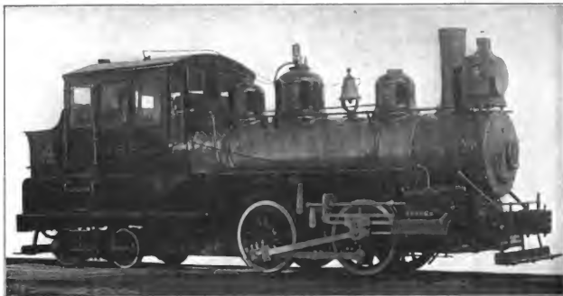
Fig. 11. Forney Four-Coupled (0—4—4) Locomotive with Four-Wheel Rear Truck. Built by the American Locomotive Co. Cylinders 17 in. x 24 in., Working Steam Pressure 165 lbs. per sq. in., Total Heating Surface 1,209 sq. ft., Diameter of Drivers 50 in., Weight on Drivers 80,500 lbs., Total Weight 113,500 lbs.
